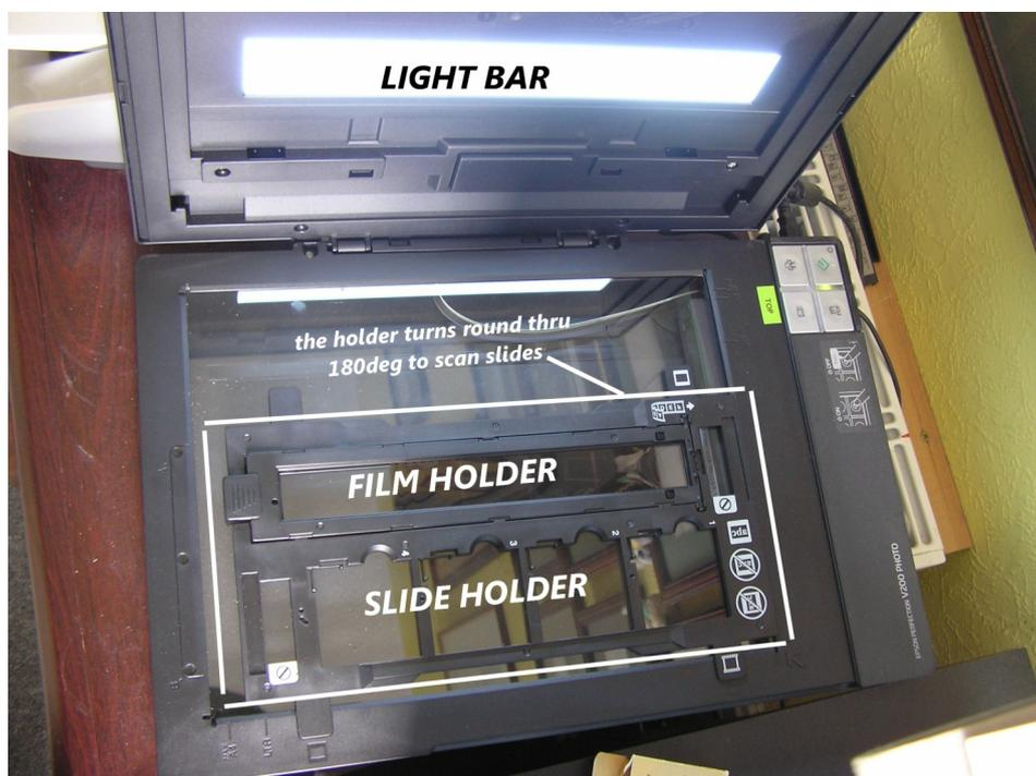
Under the lid of a normal scanner is a white plastic plate (much like a photocopier). The special scanner for film has instead a light bar under the lid that shines light through the film of the negative or transparency. There is a plastic holder that holds the film in place (see picture on previous page).
